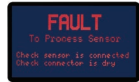
Sensor Probe Fault Screen.
