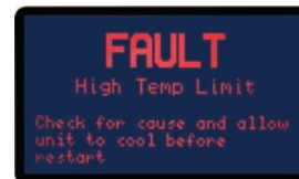
High Temp Limit Fault Screen.
