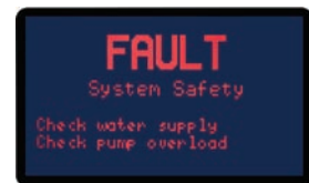
System Fault Screen. Indicates a water supply or a pump overload fault.
