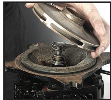
Aligning impeller and spring
