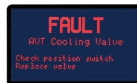
AVT Valve Fault Screen.
