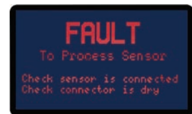
Sensor Probe Fault Screen.
