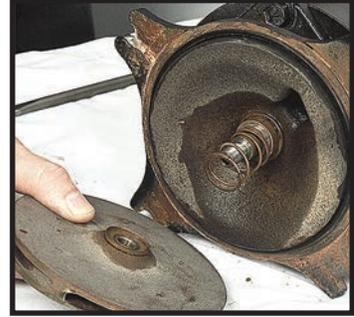
Seal components Figure 5.1I
