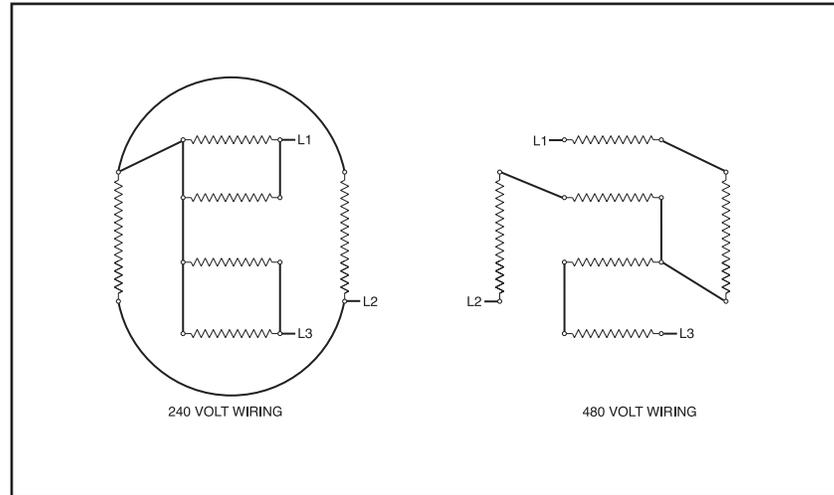
Wiring schematics for 240 and 480 volt heaters Revised 4/11
