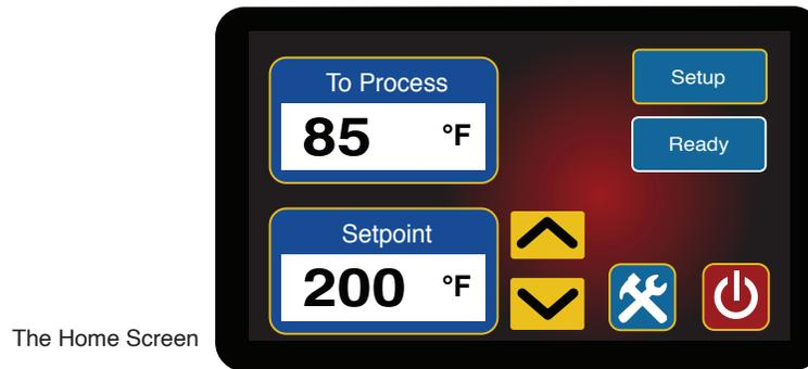
1. The Home Screen is the screen that appears once the unit has started. It offers To Process temperature, Setpoint temperature, Setup button, the Tools and Status button and various machine and alert icons.
