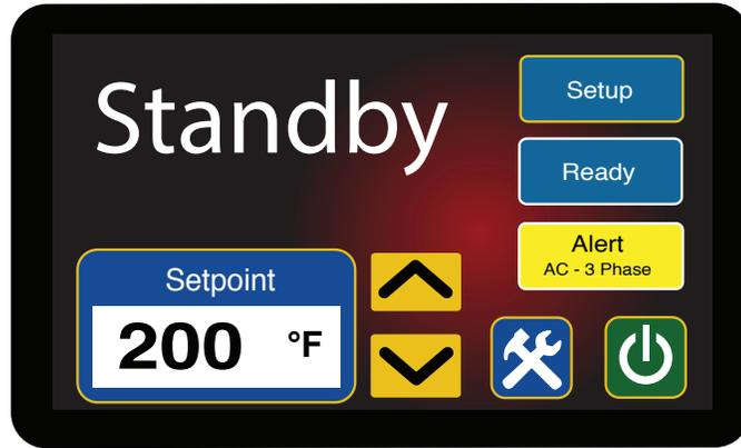
1. **Phase:** Follow the procedure outlined in section 3.2. paragraph B 'Electric Motor Phasing' to correct a phase error. If a phase error can not be cleared even though the pump motor is rotating correctly, the three phase monitor is defective and should be replaced. Disconnect the unit until a replacement is obtained.
