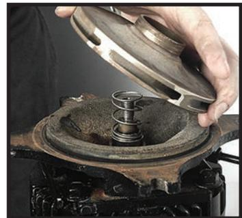
Aligning impeller and spring Figure 5.1L
