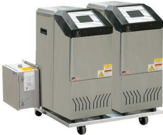
Molders often need to run different temperatures on each mold half to produce the best quality part.
