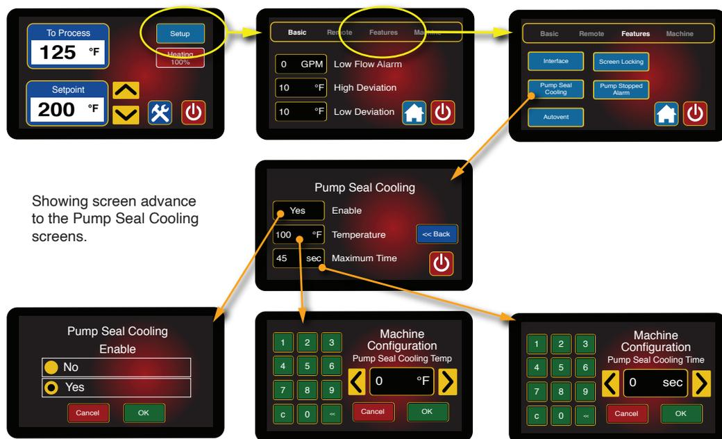
1. Pump seal cooling is a feature to automatically cool the unit before shut down, after the user has pressed the red Shut Down button.
