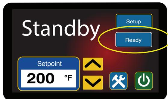
2. **Ready.** When the electrical power supply is engaged the display will illuminate. The Standby Screen is displayed and shows the last selected Setpoint temperature. The Ready Indicator is shown if the unit is ready for operations. The Setup, Tools & Status and Power buttons are also displayed.
