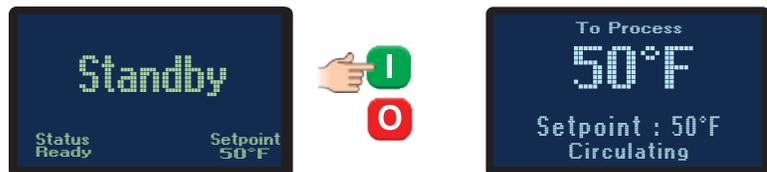
4. To select setpoint temperature, press and hold the Up or Down Arrow keys until the desired setpoint temperature is displayed in the display window. The default range for the setpoint temperature is 48°F - 90°F or 9° - 32°C.
