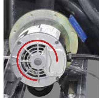
Correct shaft rotation is clockwise.
