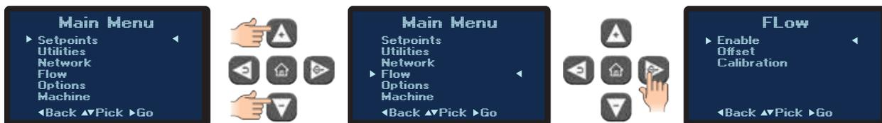
**B.** Advance to the Flow Enable / Disable screen. Select Enabled to enable the flow option.
