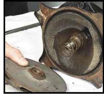
Seal components Figure 5.5H
