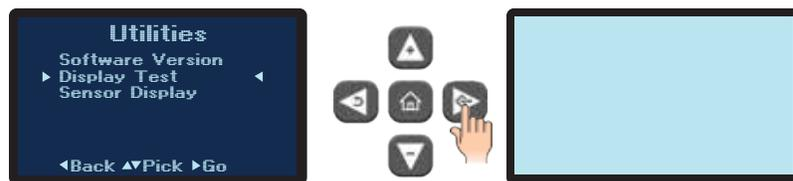
1. Select the Display Test item from the Utilities Menu to advance to the Display Test screen.
