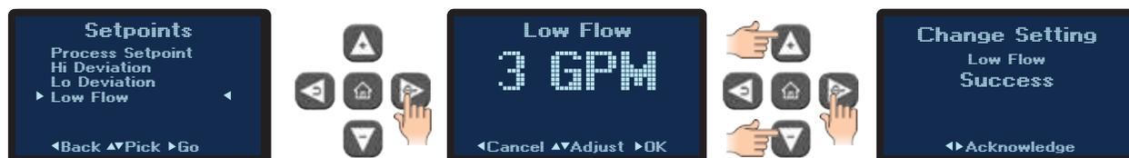
1. The factory default is 0 GPM. The range for the Low Flow is from 0 to 100 GPM.
