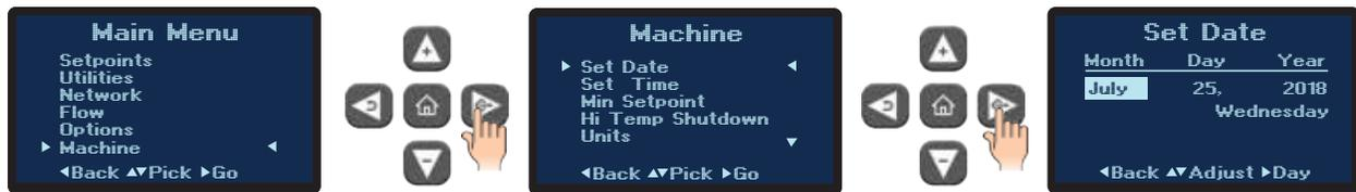
1. Set the date by selecting the Set Date option from the Machine Menu. Using the Up and Down Arrow keys to select the month, day and year. Use the Select and Back Buttons to advance between Month, Day and Year.
