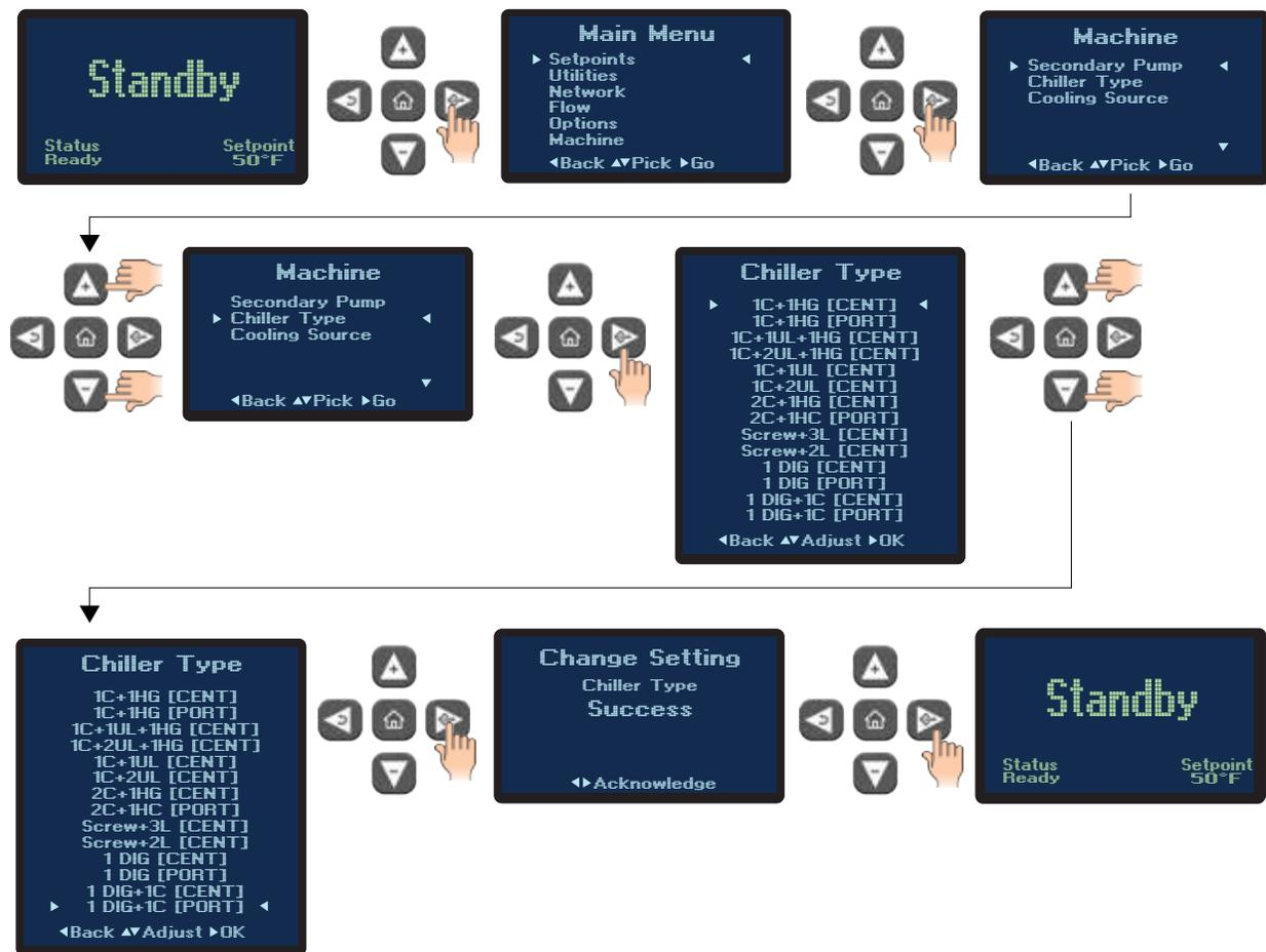
2. On the MG control instrument, press 'Machine'.
