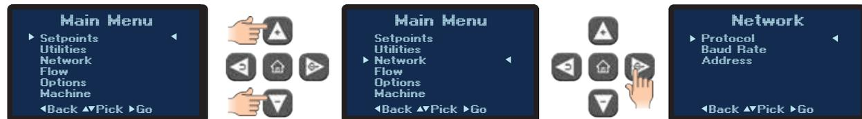
B. **Protocol:** This is the data format for communication between the unit and the host computer. Available values are SPI CCP, Modbus RTU and CAMAC. SPI is the standard Society of Plastics Industry, Inc. protocol. CAC is the CAMAC protocol used on older Milacron machines. Modbus RTU is used in serial communication and is a common serial communications protocol for industrial equipment.
