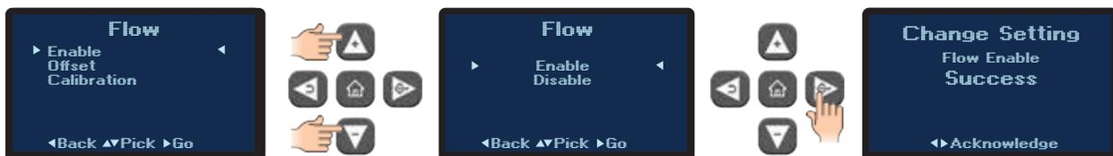
**C. Offset.** This allows the user to select the flow offset according to the pump horsepower.
