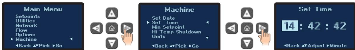
1. Set the time by selecting the Set Time option from the Machine Menu. Using the Up and Down Arrow keys to select the hour, minute and seconds. Use the Select and Back Buttons to advance between Hour, Minute and Seconds.
