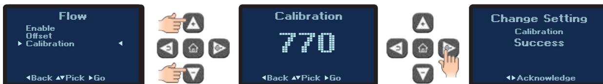
1. Using a reliable and accurate external flow meter the user can input a calibration constant value in the screen so that the unit flow display matches the external flow meter.
