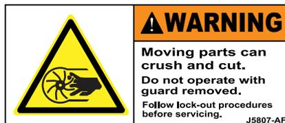
Alerts user to the danger of the rotating condenser fans on air condensed units.
