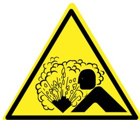
This symbol is seen on all chillers to alert user to the danger of the refrigeration system under pressure. System should only be serviced by a licensed technician.
