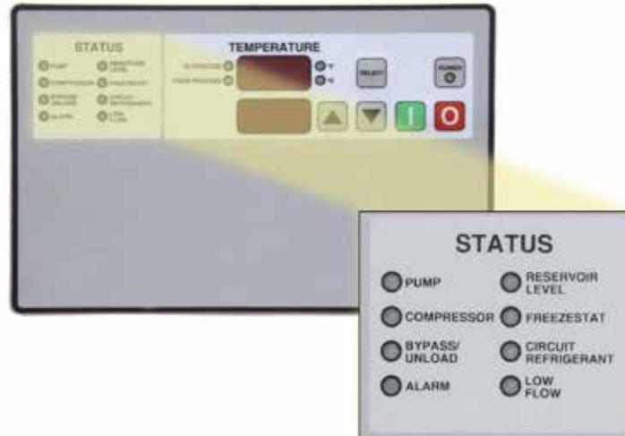
4. **ALARM:** Illuminates 'solid red' when the "to process" temperature has deviated +/- 10° from setpoint. Note: The temperature deviation alarm circuit is only activated after the chiller has cooled the circulating fluid to the setpoint one time.
