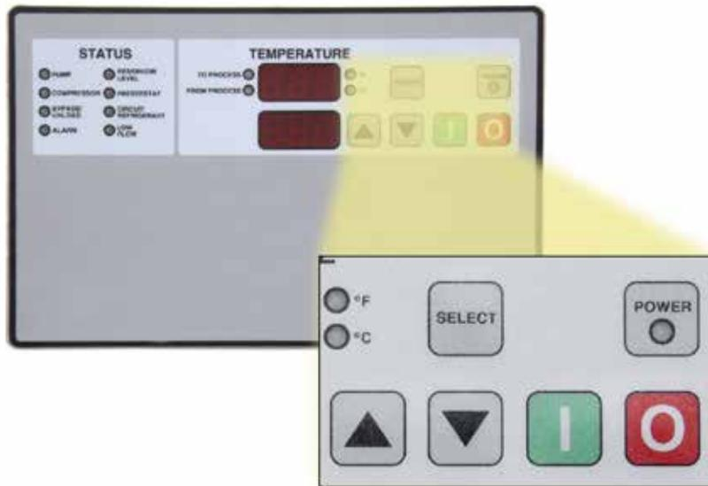
1. **START:** (green color button) this push button engages/disengages electrical supply to the coolant pump and refrigerant compressor. Please note that the refrigerant compressor will not start unless the coolant pump is operating.
