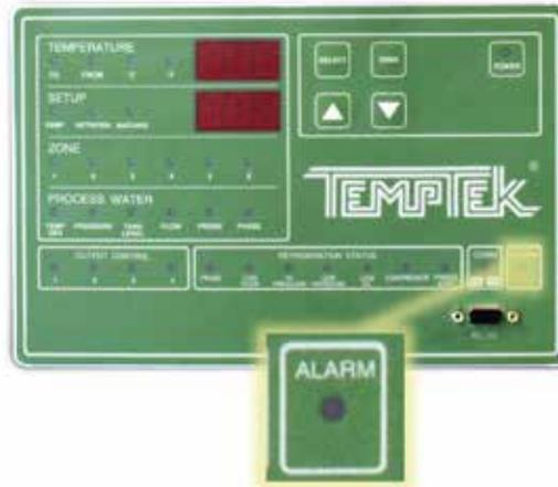
1. When this light illuminates RED, an unacceptable condition has developed, at which time a 115 volt alarm output is generated for an external (factory or customer installed) alarm beacon or buzzer.
