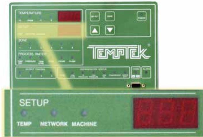
1. When the **SELECT** key is pressed, and the unit is NOT in zone display the display will cycle forward through all available temperature and setup parameters. The currently selected setup parameter is indicated in the **TEMPERATURE** display window (i.e. “Hi” for High Deviation, “Lo” for Low Deviation) and the value is displayed in the **SETUP** display window. Values are changed with the **Up** and **Down** arrows. The available parameters are listed below:
