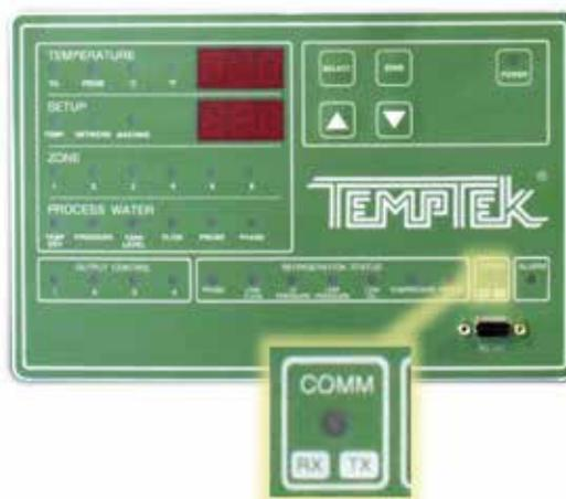
1. The communication display indicates the type of (SPI/CAC) exchange between the host computer and the controller.
