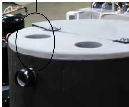
Typical reservoir lid and From Process opening.
