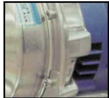
Typical pump casing bolt
