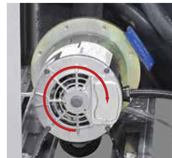
Correct shaft rotation is clockwise.
