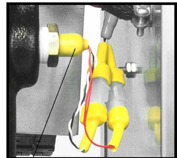
Sensor probe and high temperature limit
