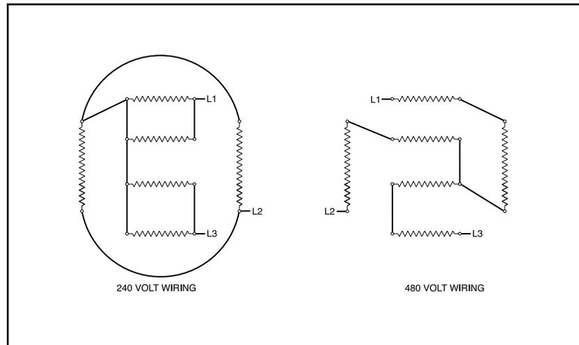
Wiring schematics for 240 and 480 volt heaters
