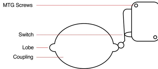
NOTE: Important... the valve stem should be in this position (as indicated in the diagram) and the valve should be CLOSED. If the valve is open, manually turn the square stem 90° so that the valve is closed.
