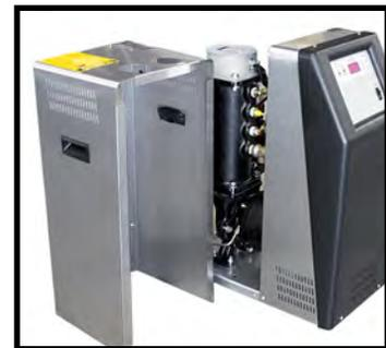
Remove lift-off access panel      Figure 5.1B
