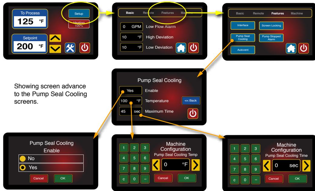
2. For example, if the unit is operating at a high temperature and the user presses the red Shut Down button, the unit will continue to operate in the cooling mode until the Pump Seal Cooling Temperature is reached or the Pump Seal Cooling Time has elapsed.
