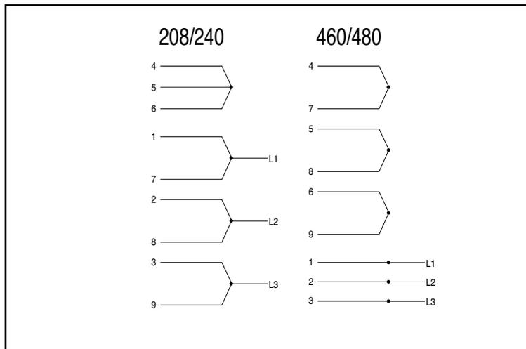
Wiring schematics for 240 and 480 volt pump motors Figure 5.5C
