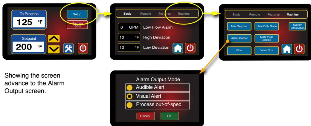
Showing the screen advance to the Alarm Output screen.
