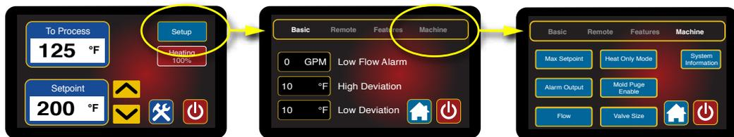
Showing the screen advance to the Machine Setup screen.
