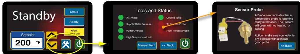
Showing the screen advance to the Sensor Probe screen.
