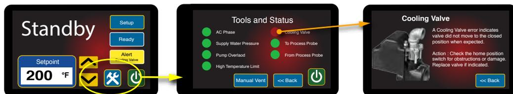
Showing the screen advance to the Cooling Valve screen.
