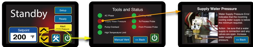
Showing the screen advance to the Supply Water Pressure screen.
