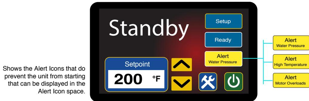
1. **Water supply pressure inadequate.** The Alert - Water Pressure icon is displayed. The unit can not operate without adequate water supply pressure. Sufficient water supply pressure must be present to close the water pressure switch. See section 2.3 for additional information.
