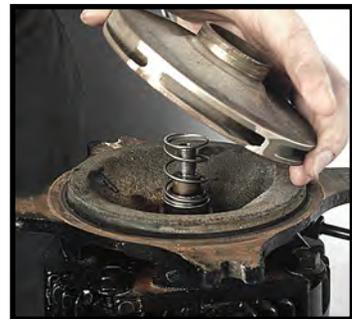
Aligning impeller and spring Figure 5.1L
