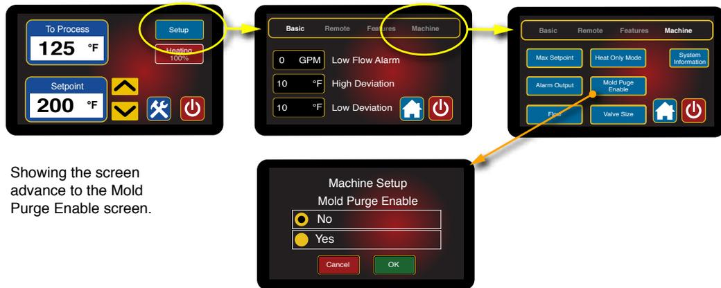
1. Select Yes to enable the Mold Purge system. Then press OK to save the selection and return to the Machine Setup screen. Press Cancel to return to the Machine Setup screen without saving the new value.
