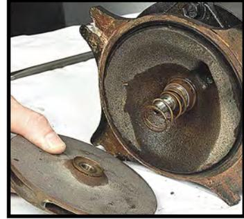
Seal components Figure 5.1I
