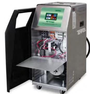
Thermoformed panel removed and electrical cabinet open. Figure 5.5A
