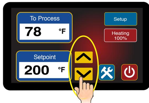
2. **Press the Setpoint window.** The gold outline around the window indicates the window can be pressed to advance to another screen.
