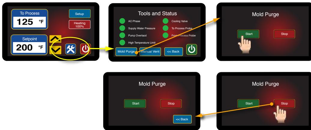
5. Press the Stop button to disengage the purge cycle. Use the Back button to return to the Tools & Status screen.
