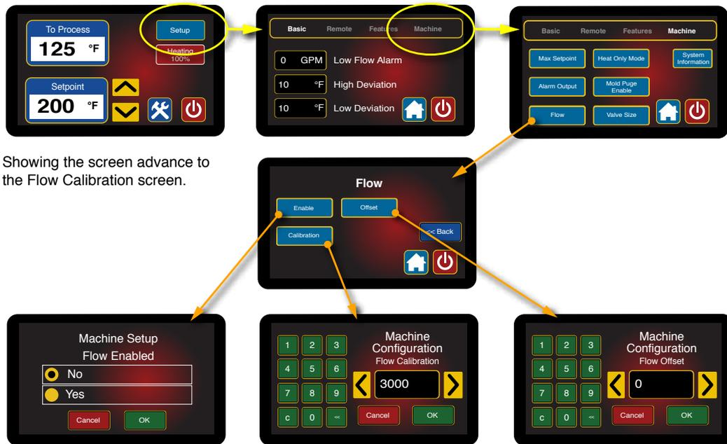
Showing the screen advance to the Flow Calibration screen.
