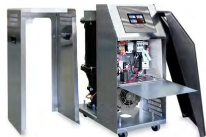
Thermoformed panel removed and electrical cabinet open.      Figure 5.1C
